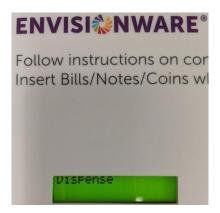
**Step 3.** Tap the **RIGHT** button and LCD display should indicate the denomination (possibly nickels) and quantity. Press **ENTER** to dispense. Our example shows that we already have zero nickels in the nickel tube. You have two options now to zero out the tubes.
