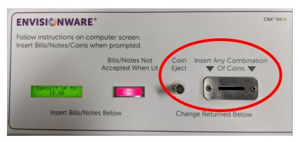
**Step 4.** When you have inserted to the desired amount (recommend to fill at least half way for each tube) press the **LEFT** button to go back to "Load Change" or press the **RESET** button.
